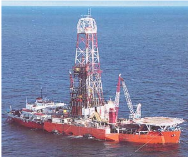
Figure 3-2: Northern Explorer II (formerly the Canmar Explorer II and Explorer II), Drill Ship (Ref. /13/)
