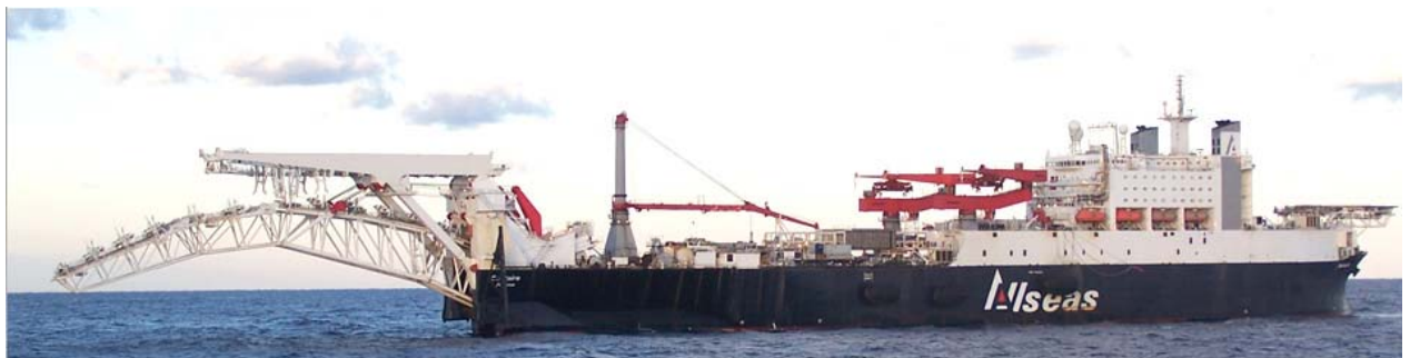
Figure 5-3: Pipe Lay Barge, Allseas Solitaire (Ref. /44/)
