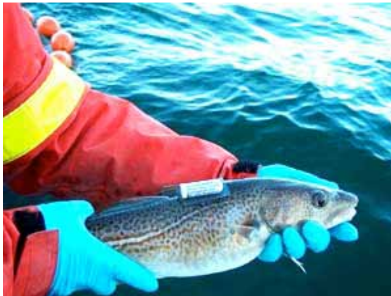
Figure 10. An archival (data storage) tag attached to a cod. Image from Star-Oddi website
