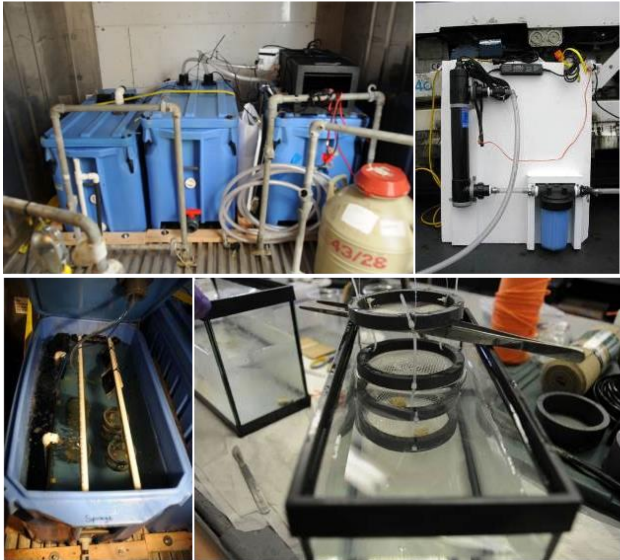
Figure 10. Clockwise from the top left: Tank setup in the refrigerated container; filter housing and UV setup; sponge fragments in culture array; fragment culture arrays in tank..
