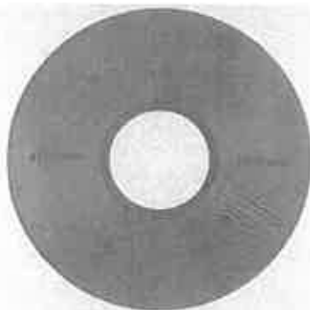
Figure 4. A read-only CD with scratches on the top side of the disc. When the laser light encounters this damage in the metal layer it will shine right through the disc rather than being reflected back to the detector. Therefore no signal will be created, and the disc will not play properly.
