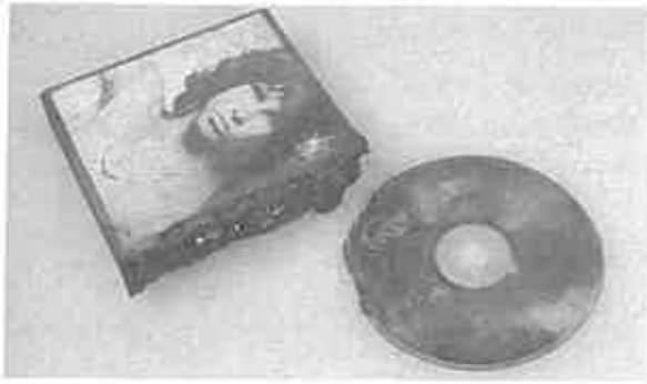
Figure 15. Serious damage can result when CDs are subjected to extreme heat, e.g. from a fire.
