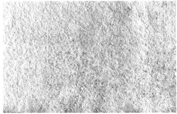
Fig. 4 Detail showing pronounced texture from drying felts in antique papers.
