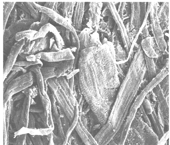
Fig. 5 Scanning electron microscope (SEM) image of China paper, 450X. Delacroix (BMA 1925.12.1).
