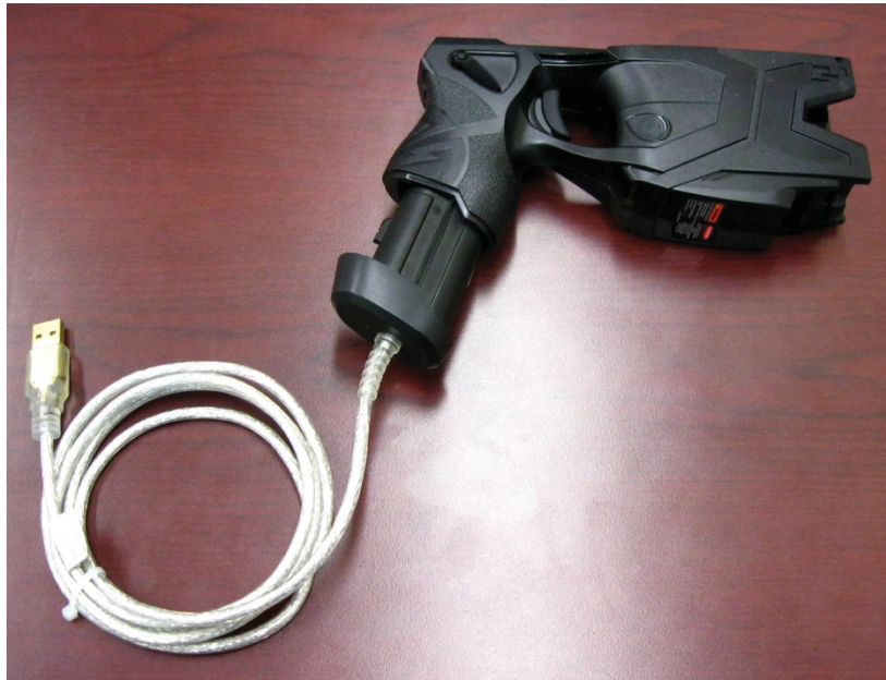
Figure 20: USB adapter partially inserted into the Taser X2 grip
