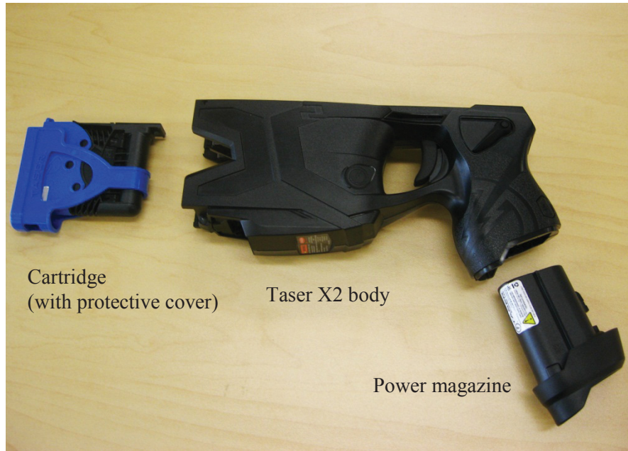
Figure 1: The three main parts of a Taser X2
