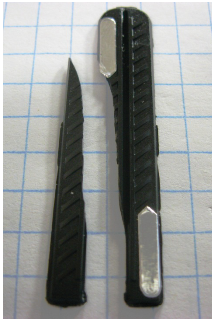
Figure 44: Irregular separation of the blast doors
