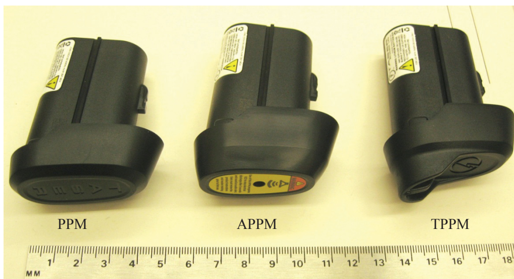
Figure 15: Three different Taser X2 PPM models viewed from the side
