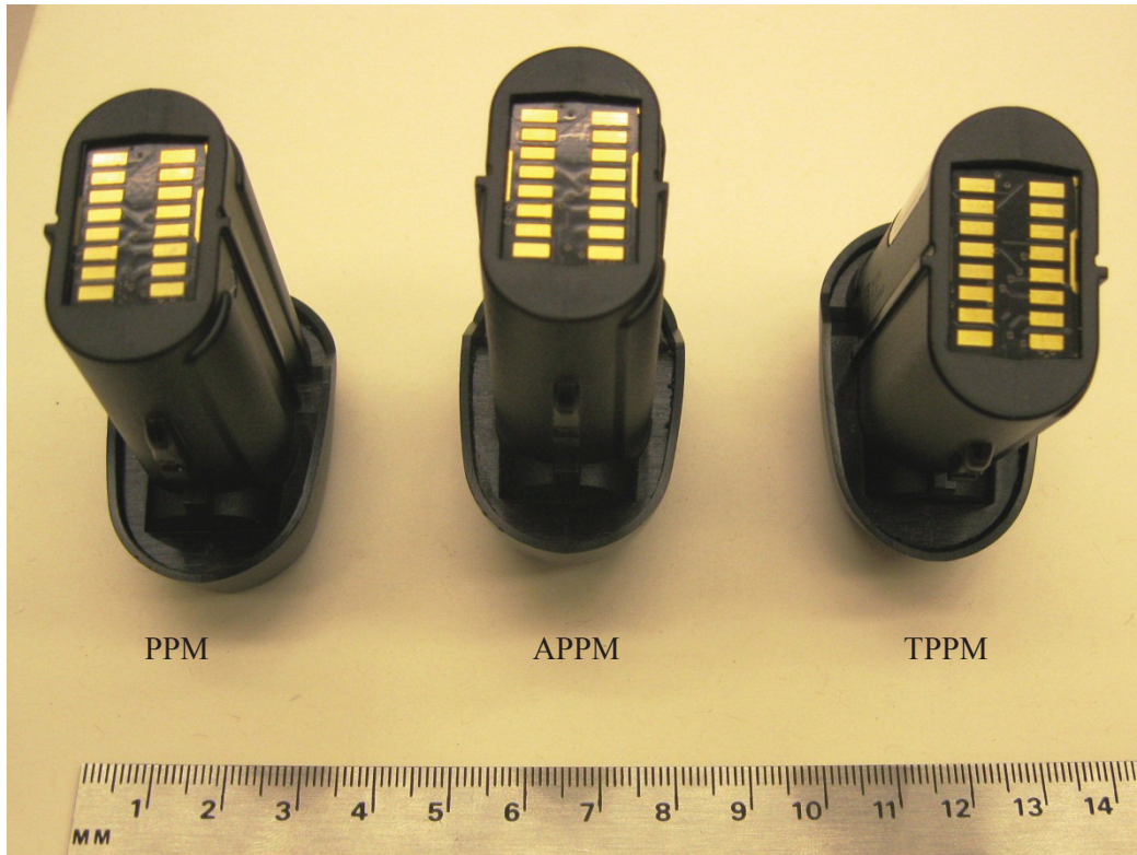
Figure 17: Contact pads on the PPMs
