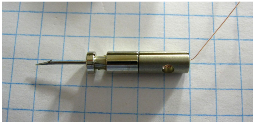
Figure 13: Smart Cartridge probe
