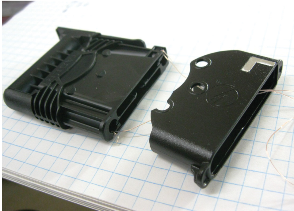
Figure 47: Taser X2 cartridge separated into two parts
