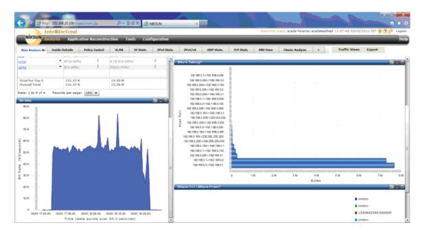
Test traffic between HMI and PLC as seen by IntelliDefender
