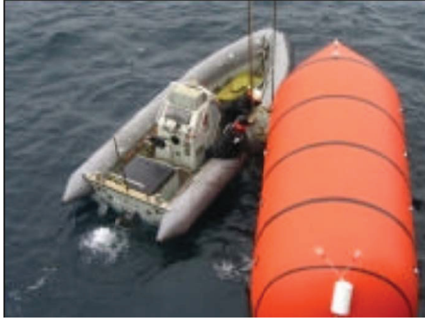
Figure 3 - Barracuda USV (left) and HSITT (right) [1]
