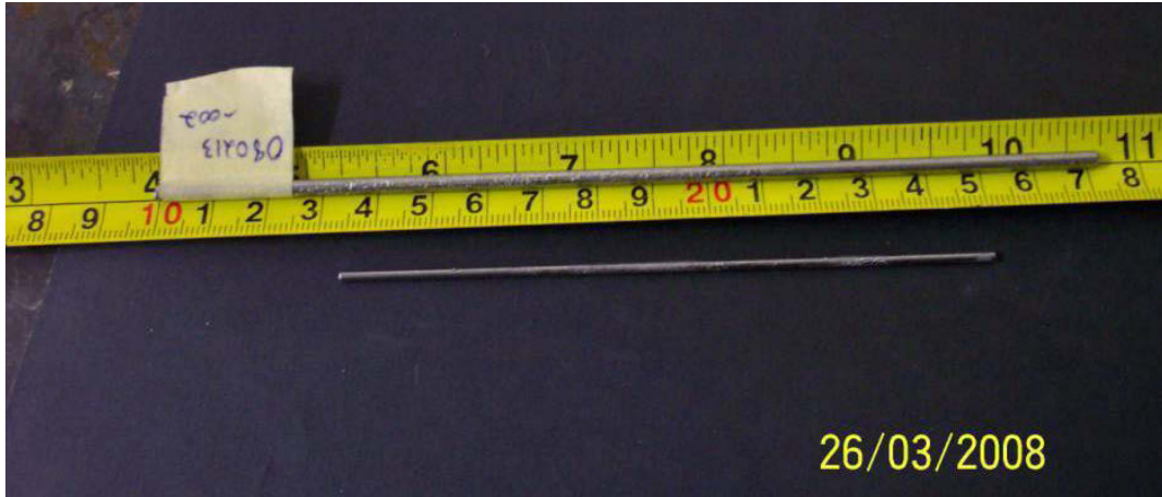
Figure 3: Fe-Ga suction cast rods. The smaller rod is about 1.9 mm in diameter and 12 cm long and the larger rod is about 3.2 mm in diameter and 17 cm long.
