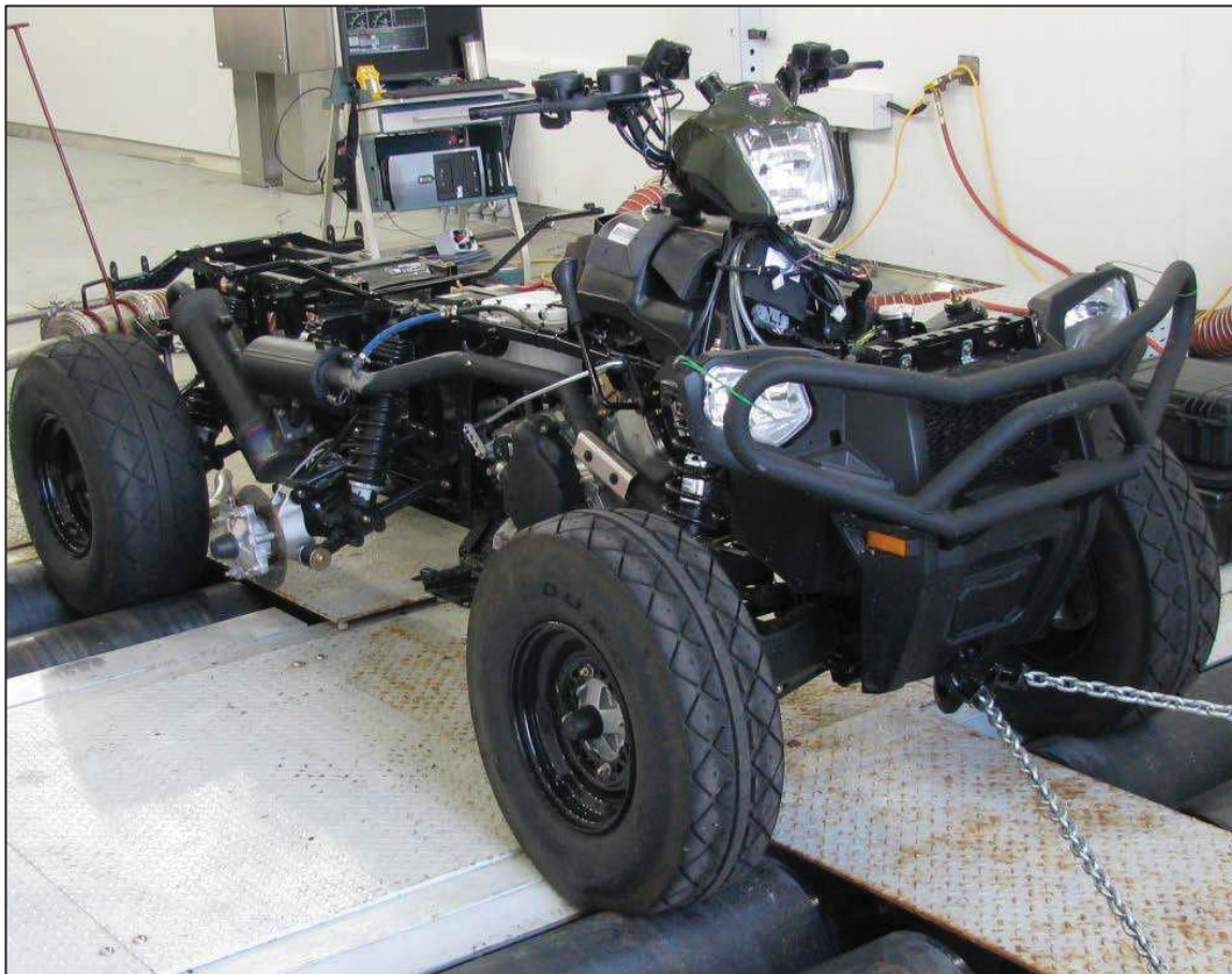
Figure 1: ATV with bodywork removed, on chassis dynamometer.
