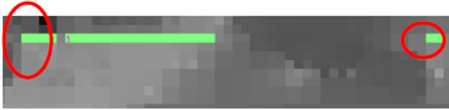
Figure 3-11: Inset circles show the pixels which will be in contact with the water drop, considering a fixed penetration, but do not contribute towards line parameters as they are less than 5 conjoined pixels.
