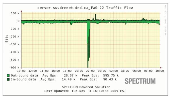
Figure 7: JNDMS Integration Server Bandwidth Utilization over a 24 hour period
