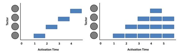
*Figure 5. Left - "Up" activation sequence for the "sequential" display. Right - "Up-Down" pattern of activation for the "equalizer" display.*
