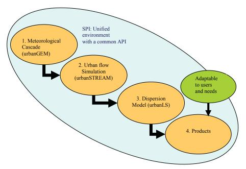
Figure 1: Schematic of the CUDM system.
