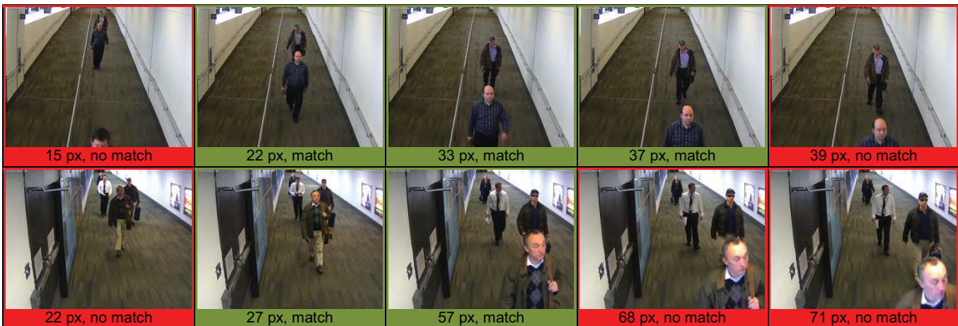
Figure 31 – Sharpness in CCTV camera
