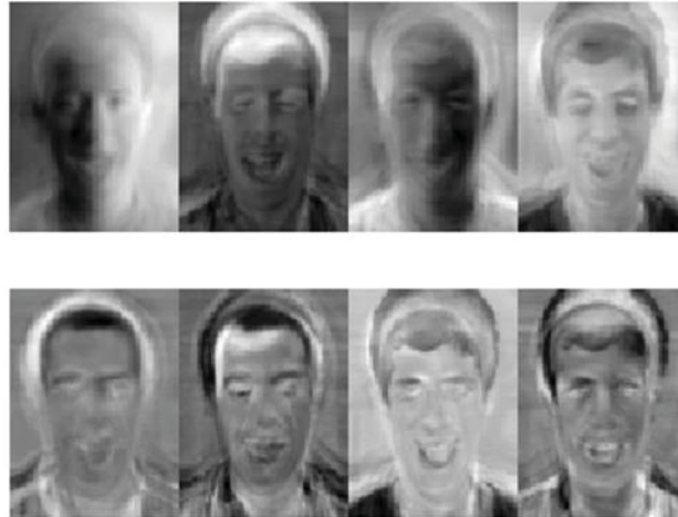
Figure 2-5 Top: Eigenfaces (PCA), Bottom: Fisherfaces (LDA) (Source: [P-1])
