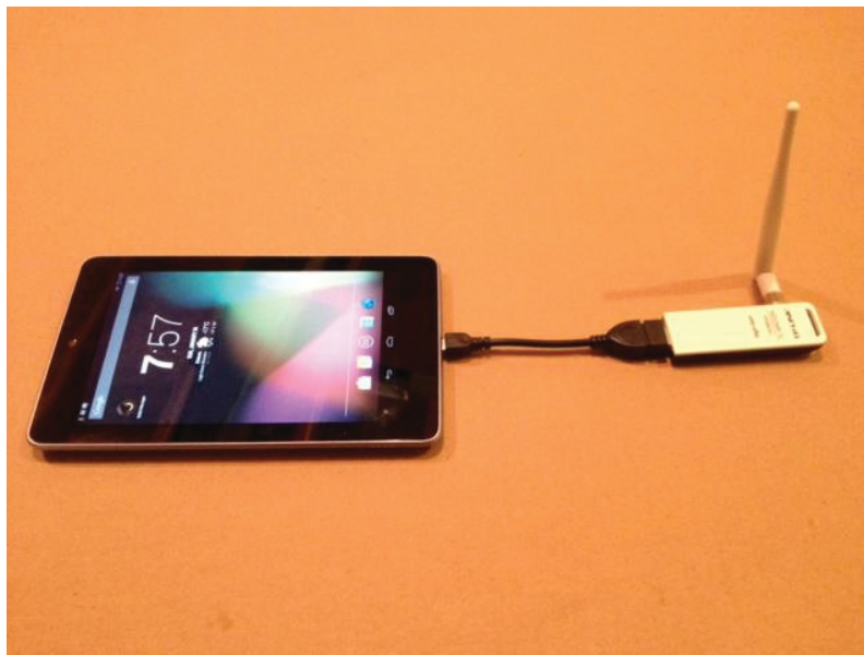
Figure 16: Google Nexus 7 and External TP-link Wi-Fi Radio
