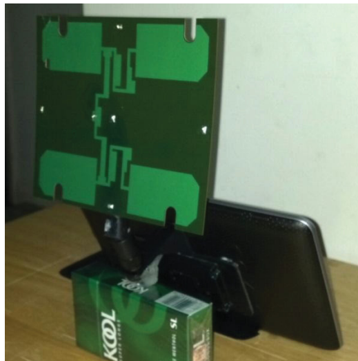
Figure 5: A Tablet with a Long Range Directional Antenna
