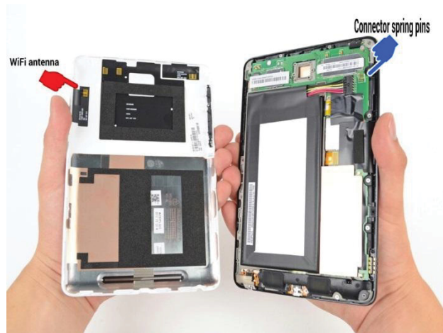
Figure 4: External Antenna Hardware Modifications
