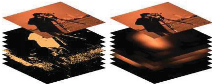
Figure 3. Distribution Fields explode an image into multiple layers, one for each histogram bin. These layers are shown on the left, and shown spatially smoothed on the right.
