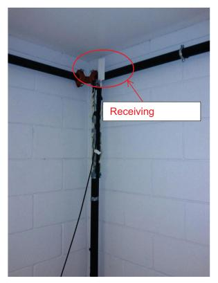
Figure 4-26: Receiving antenna placed in the corner of the room
