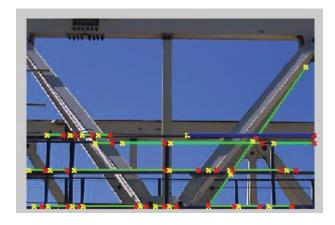
Figure 3-24 Hough lines mapped back into image with starting and stopping positions
