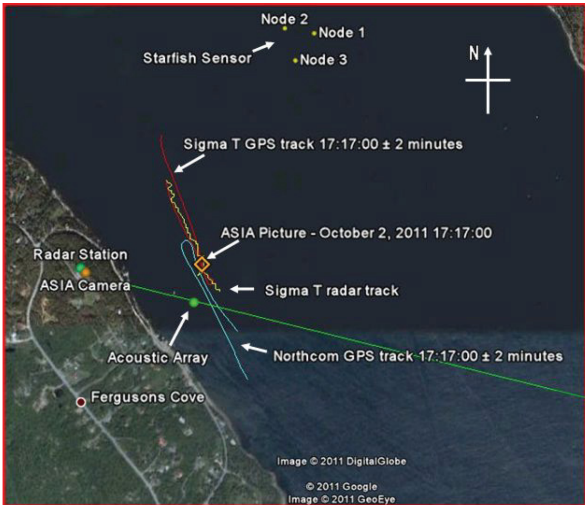
Figure 3: The SICCPA trial vessel tracks based on GPS and radar. The physical deployment of ASIA, radar and the acoustic array are also shown.
