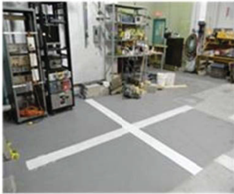
Area cleared, floorpainted, coordinate system laid down.
