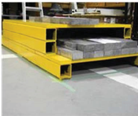
Second layer of lead installed.
