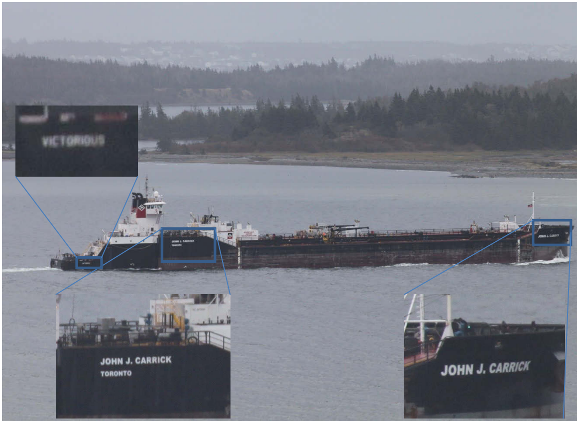
Figure 38: In this figure, an operator might well imagine that this vessel is the JOHN J CARRICK because of the name printed on the side and bow. AIS, however, identifies this ship as the VICTORIOUS (and so ASIA associates this name with the ship). The discrepancy has an innocent explanation because the ship also shows the name VICTORIOUS, somewhat inconspicuously, in very small letters near the stern.
