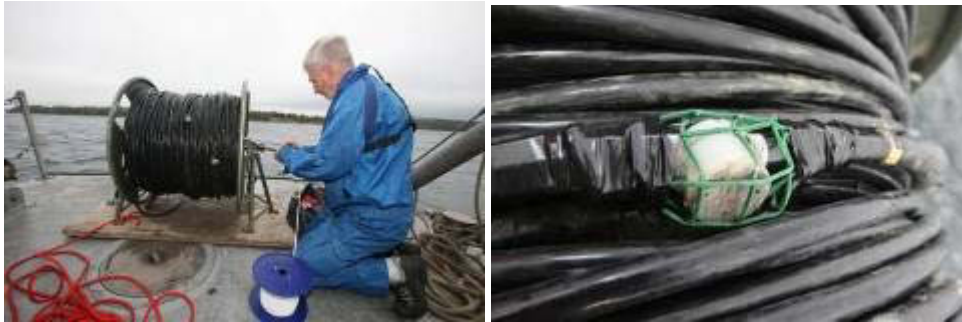
Figure 7: Configuration of the electrode system and a picture of a single electrode element mounted on the cable. The total electrode system contains 16 silver/silver chloride electrodes, which form 8 electrode pairs. The distance between the electrodes in an electrode pair is 25 m and the distance between consecutive electrode pairs is 0.6 m.
