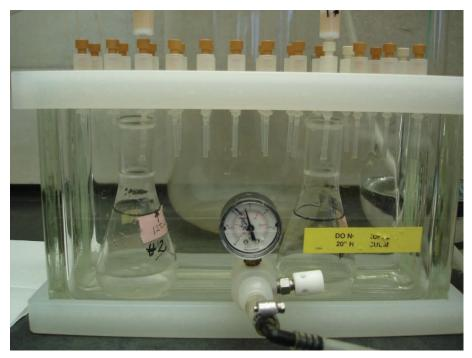
Figure 2: Collection of the effluent in 125 mL Erlenmeyer flasks
