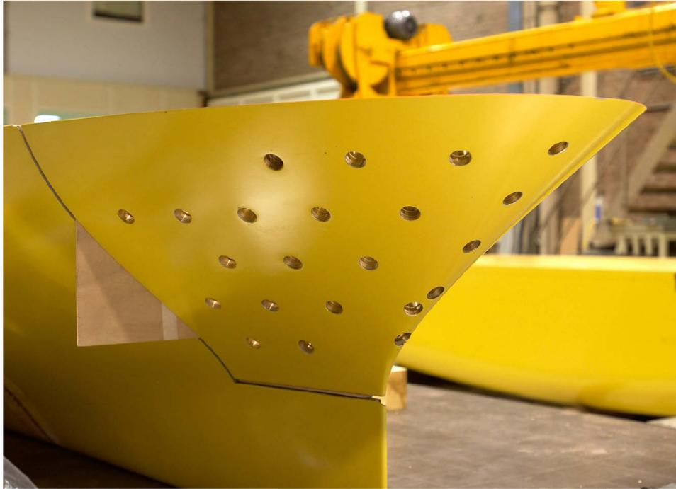
**Figure 2:** ELAST ferry model showing bow segment and pressure transducers
