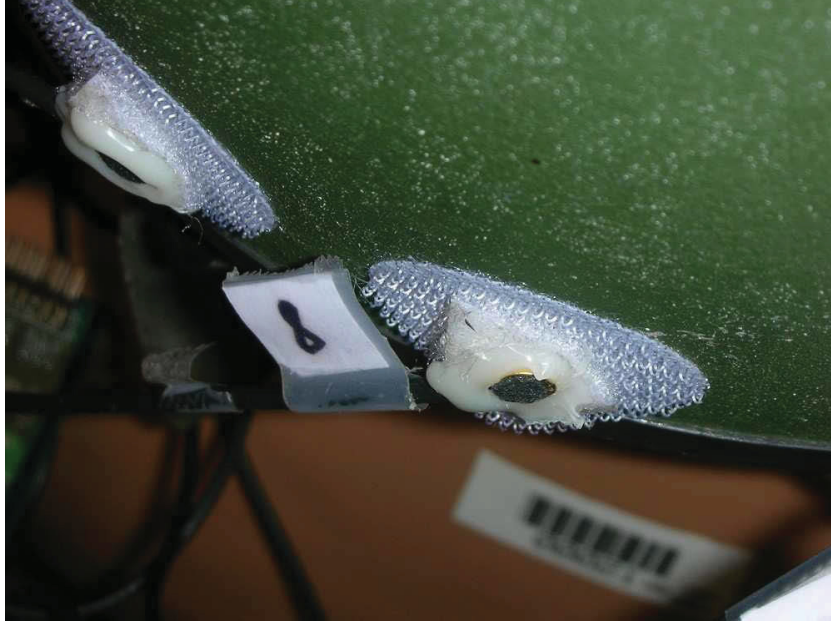
Figure 12: Detail of sensor mounting on LAP prototype. The microphone is not flat, resulting in skewed angular coverage.
