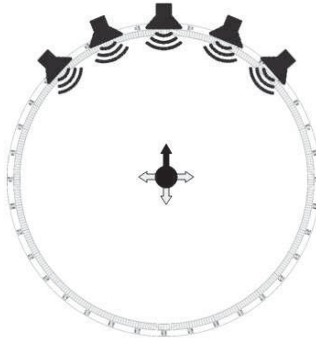
Figure 9: Loudspeaker arrangement for testing localization resolution. The black arrow indicates the helmet's initial forward direction, and the grey arrows the directions to which the helmet was rotated as the experiment proceeded.
