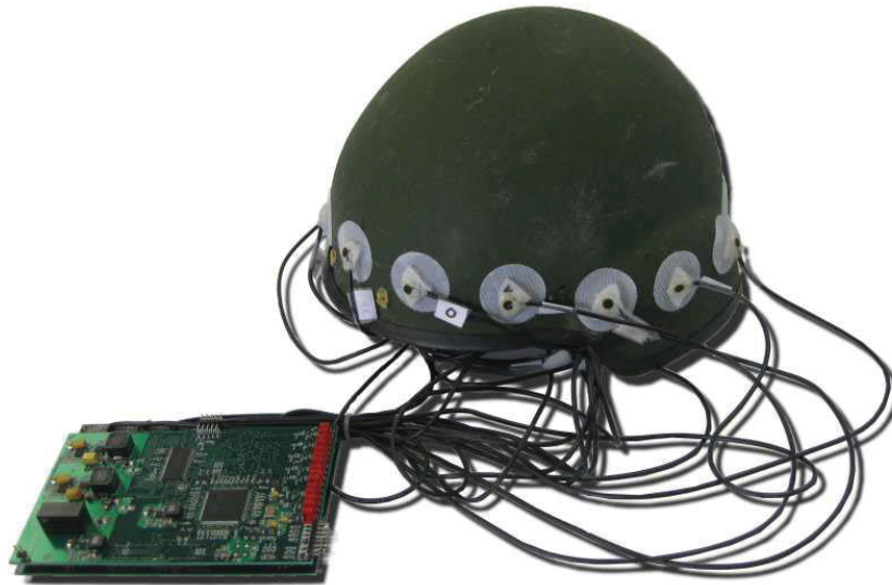
Figure 1: The Localization Array Processor (LAP) prototype, showing the helmet-mounted microphone array, the signal processing unit, and the output display.
