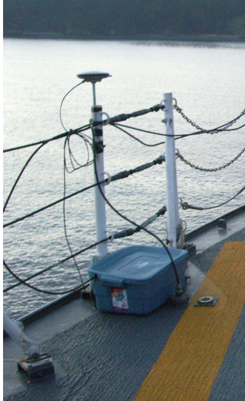
Figure 6: Example Setup for DGPS Receiver, Antenna, and Logging System
