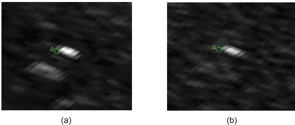
Figure 7: RADARSAT-2 data acquired on 2011-07-11: (a) HH channel; and (b) HV channel. Both AISSat-1 and MSSIS declared this ship (AISSat-1 (green square) and MSSIS (yellow triangle)) RADARSAT-2 Data and Products © MacDONALD, DETTWILER AND ASSOCIATES LTD. (2011) - All Rights Reserved..
