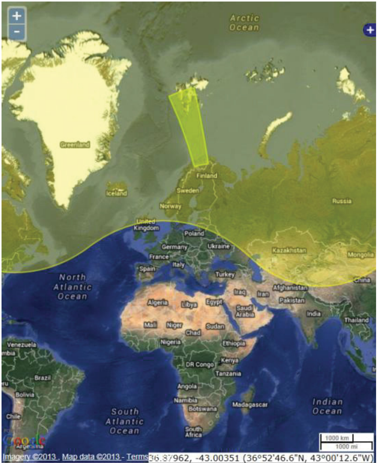
Figure A-5: RADARSAT-2 (dark yellow) and AISSat-1 (light yellow) coverage area for the 2011-06-25 collection.
