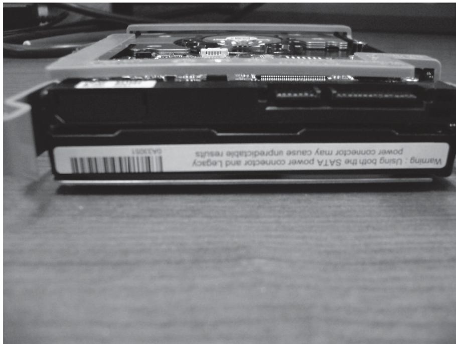
Figure 5: Side view of target disk showing disk interface
