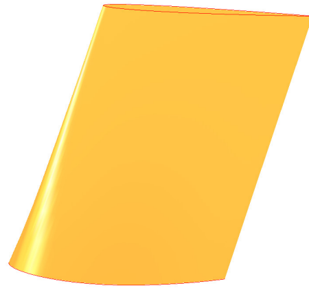
Figure 5: A surface of reference sections made from four NACA airfoils.
