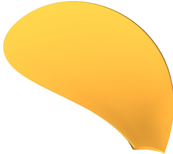
Figure 10: The blade of DTMB P4382.
