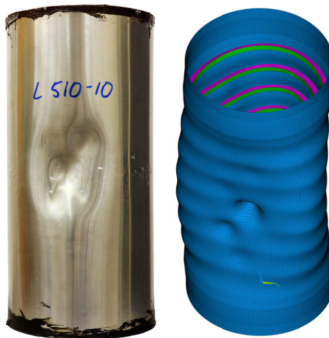
Figure 11: A photograph of specimen L510-No18 after collapse testing (left), and the collapse shape predicted using the standard FE methodology in Annex A.
