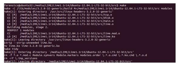
Figure 1: LiME LKM compilation under Ubuntu 12.04 x86
