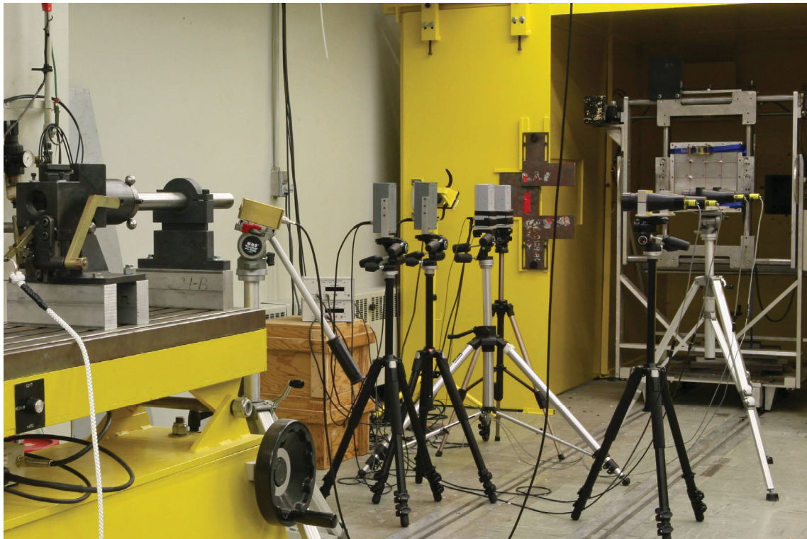
Figure 1 Setup for a test showing the gun (left), time-of-flight velocity probes and sample to be tested with a witness plate (right)
