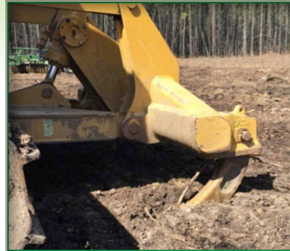
Figure 4b. Straight ripper shanks in the outside pocket of a multi-shank toolbar attached to a bulldozer
