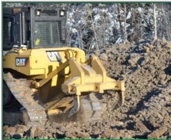
Figure 4a. Straight ripper shanks in the outside pocket of a multi-shank toolbar
