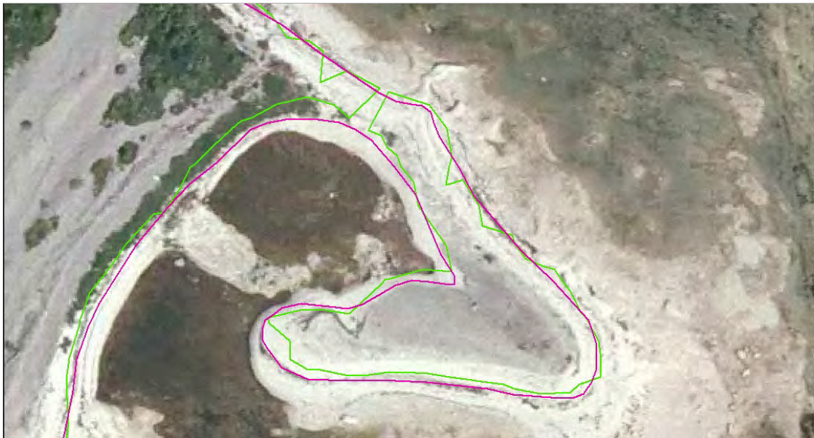
Figure 4. Differences between LIDAR (green) and photogrammetry (pink) interpretations of a water boundary
