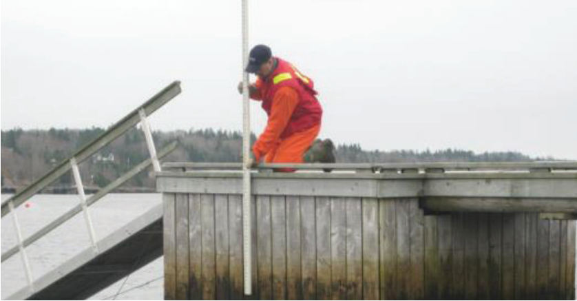
Figure 17 – Acquiring tidal bound (MHW) from wharf, NS
