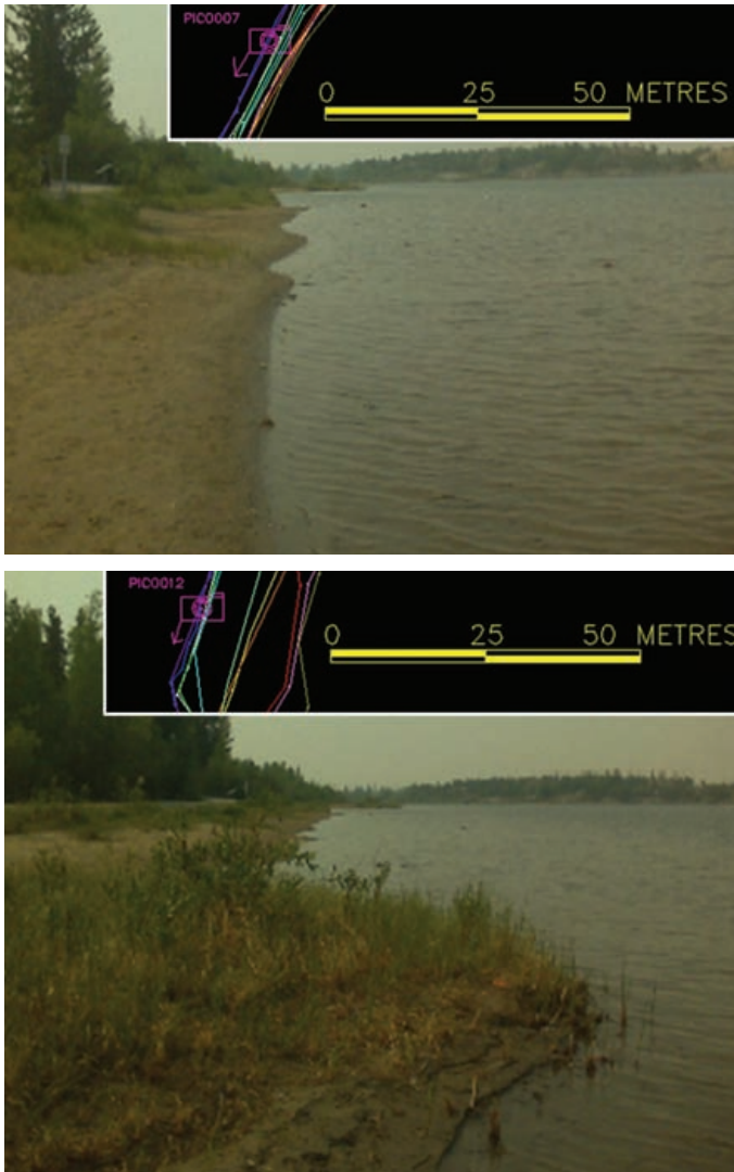
Figure 39 – Eight surveyors rendered water boundary opinions (Yellowknife, NWT): Variance of > 10m across opinions (at wide beach - bottom image); < 5m across opinions (at narrow beach - top image). June 25, 2011
