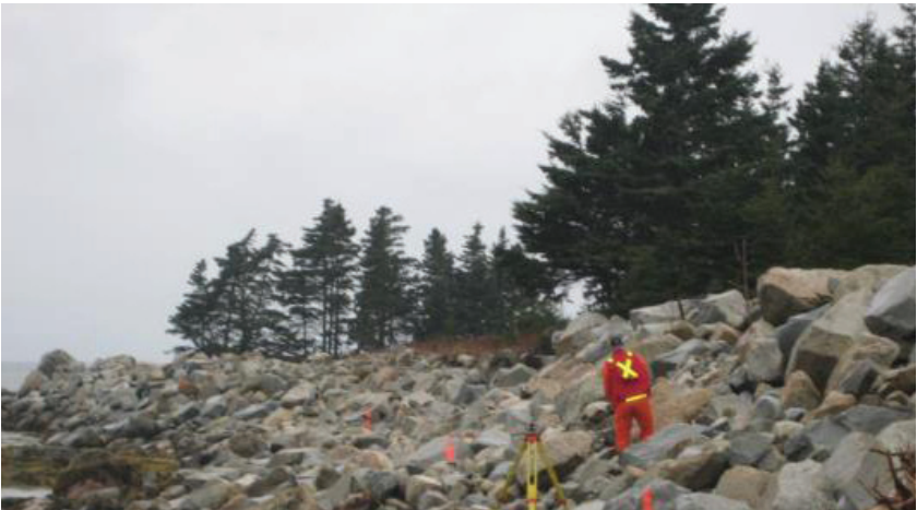
Figure 18 – Transferring tidal bound (MHW) to foreshore, NS
