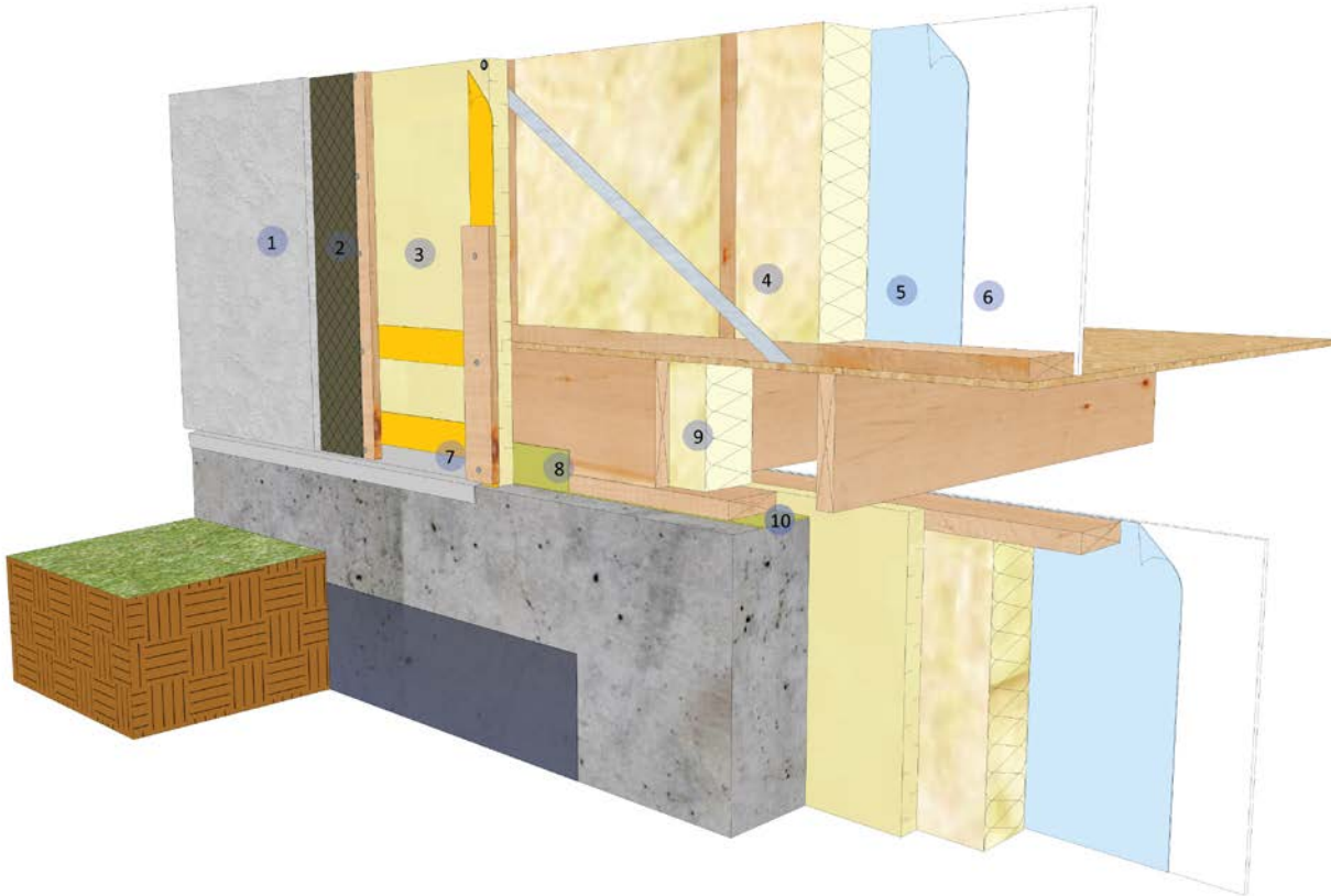
Figure 12: Illustration of a below grade wall to above grade wall transition employing exterior insulation. Illustration: Natural Resources Canada
