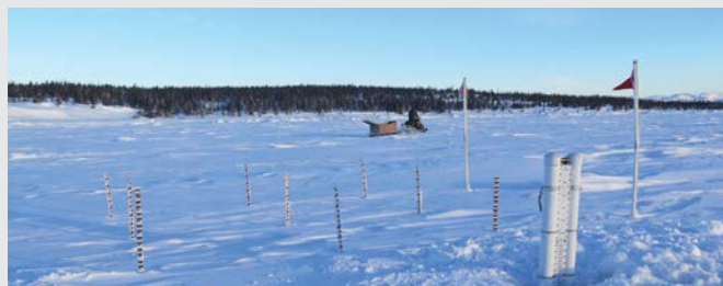
FIGURE 19: Community ice-monitoring station in Nain, NL, with a prototype SmartICE sensor frozen into the ice (right foreground). The sensor sends daily measurements of sea-ice thickness via satellite to the SmartICE data portal. Photo courtesy of R. Briggs.
