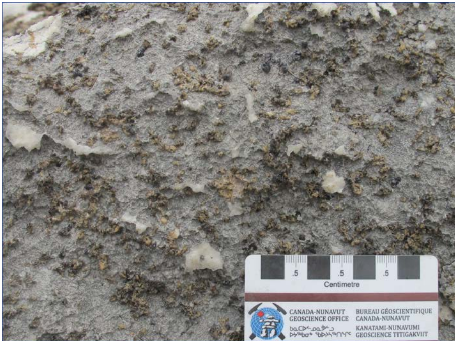
Figure 4. Impure marble (unit PLHm) from the metasedimentary sequence containing beige clinohumite crystals and aggregates of purplish-grey spinel. Photograph by H.M. Steenkamp. 2015-080
