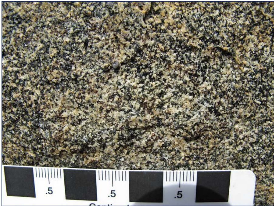
Figure 7. Example of medium-grained orthopyroxene-clinopyroxene-hornblende-biotite diorite phase of unit Pgo on western Hall Peninsula, Baffin Island, Nunavut. Photograph by M.D. Young. 2015-031
