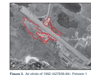
Figure 3. Air photo of 1992 (A27836-84). Polygon 1 represents a disturbed area, in units Mr and T.M. Polygon 2 represents a past beach spit in unit Mr. Polygon 3 represents a subsequent reworked area mostly in unit T.M. Polygon 4 represents an area of fill material.
