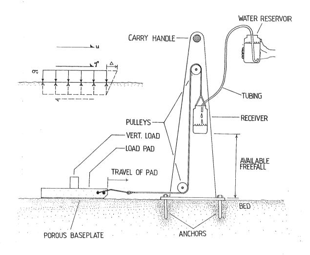
Figure 2. Diagram showing the design and operation of the INSIST device.
