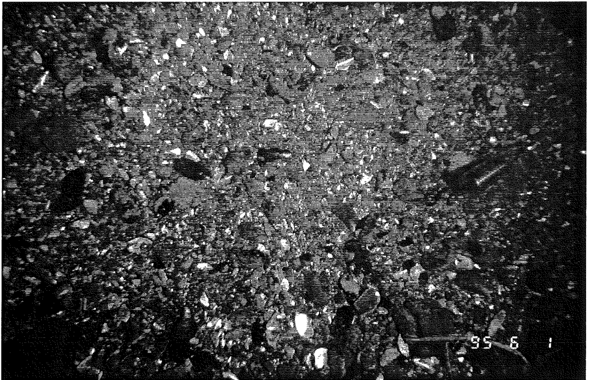
Figure 8.6.26. Seabed photographs from the centre of the Fixed Link Crossing. The seabed is composed of sorted shelly gravel, and rounded cobbles.
