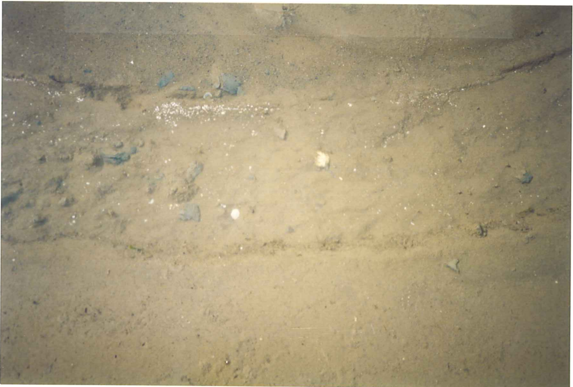
Plate 6.1.1.2. Photographs of the details of scouring left by Sea Carousel at site A. Notice the abundance of shell debris, aggregates and granules that forms a lag surface, and the undisturbed mudflat either side of the erosion scar (flow was from left to right).
