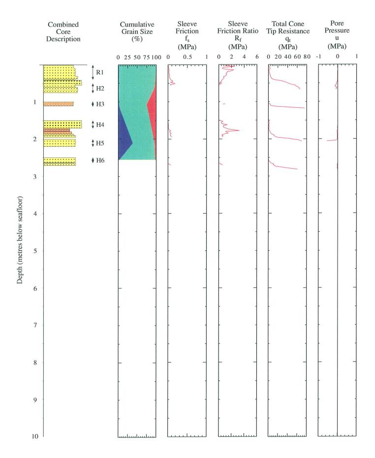
Combined Core Description Total Cone Tip Resistance Pore Sleeve Sleeve Cumulative Grain Size (%) Pressure Friction Friction Ratio qt  $\mathbf{f}_{\mathbf{s}}$  $R_{f}$ u (MPa) (MPa) (MPa) (MPa) 0 20 40 60 80 -1 0 1 0 25 50 75 100 0 0.5 1 0 2 4 6 hunhunhun . . . . . H1 H2 1 **‡** H3 **♦** H4 2 ♦ H5 H6 2 3 Depth (metres below seafloor) 4 5 6 7 8 9 10 ....l....l....l.....
