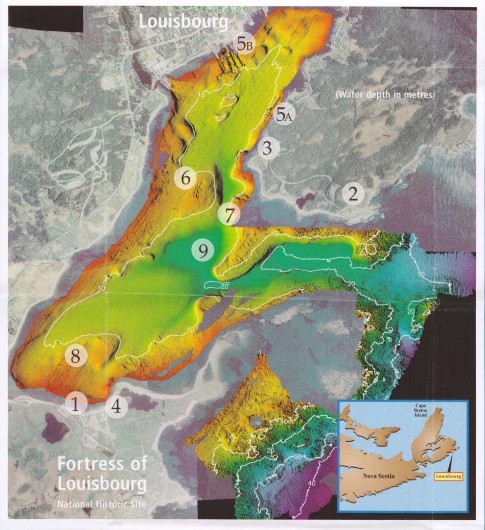
In 1996 detailed soundings of the harbour seafloor using a multibeam sonar system were completed. The soundings are combined with 1992 aerial photographs of the surrounding landscape to provide a new perspective of the Louisbourg area. The numbers in the white circles indicate the location of the adjacent images.
