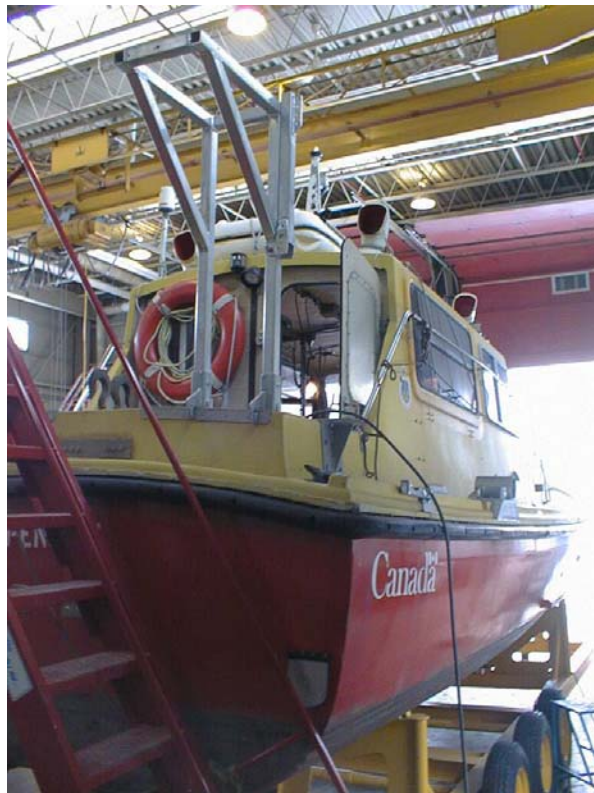
Figure 2: The stern of the Penguin showing the mount for the sound velocity profiler.
