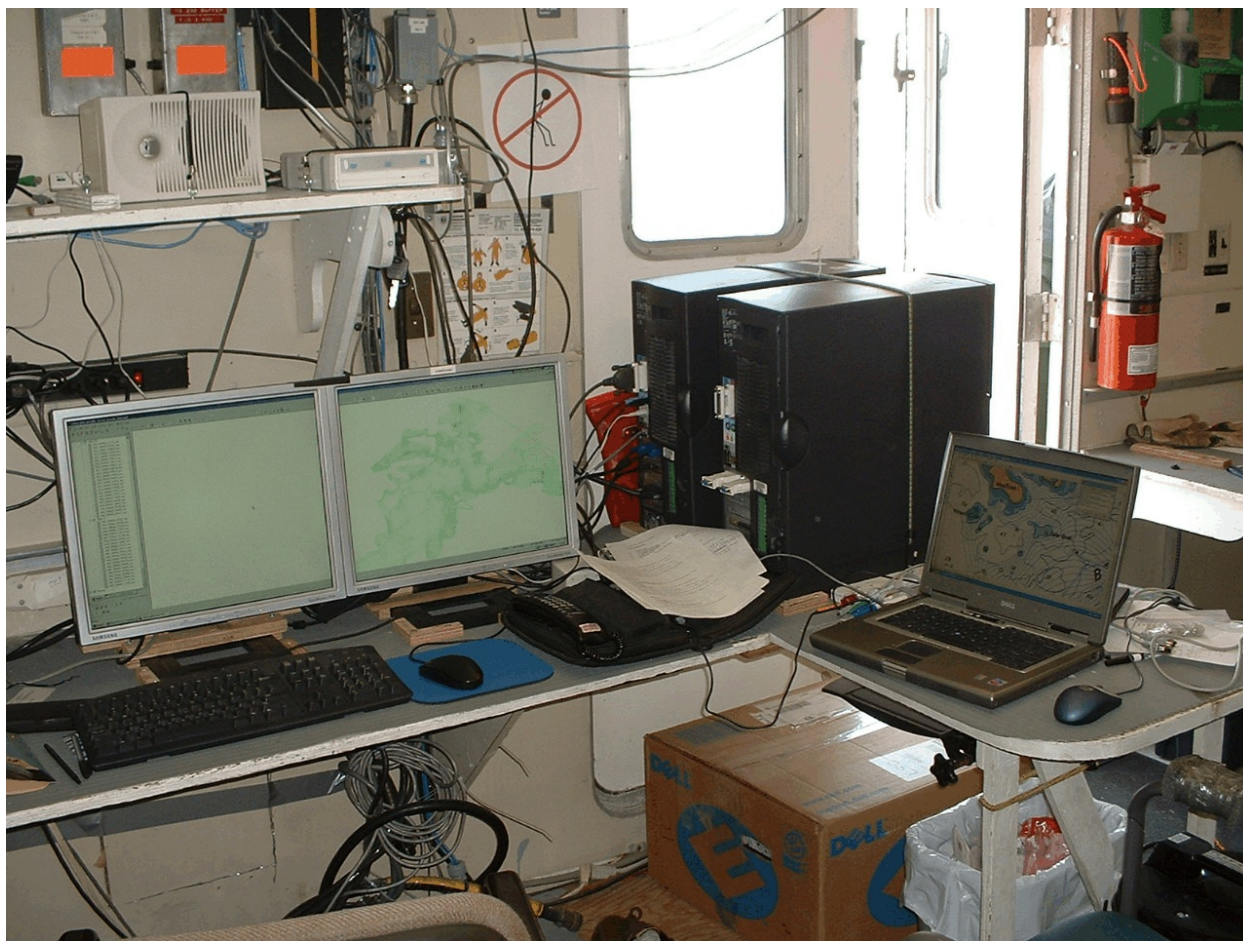
Fig. 3: The main laboratory on CCGS Creed . At left-of the image - is the 'vastraid' computer. On the desk are the twin screens and keyboard for the HIPS data cleaning system. To the right are two pcs. In the right foreground is a laptop used to write the cruise report. IT is using FUGAWI software to display a chart of the region. This program is receiving real-time navigation which is displayed on top of the chart.
