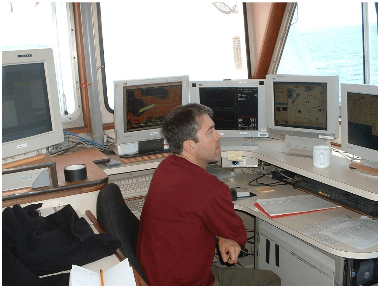
Figure 5: Setup on the bridge. At left is the MERMAID computer and screen. Next is the screen for MERLIN, then the display for the SIMRAD system. Next is the REGULUS navigation display and at the right is the PSOMV screen. Angus Robertson is seated.
