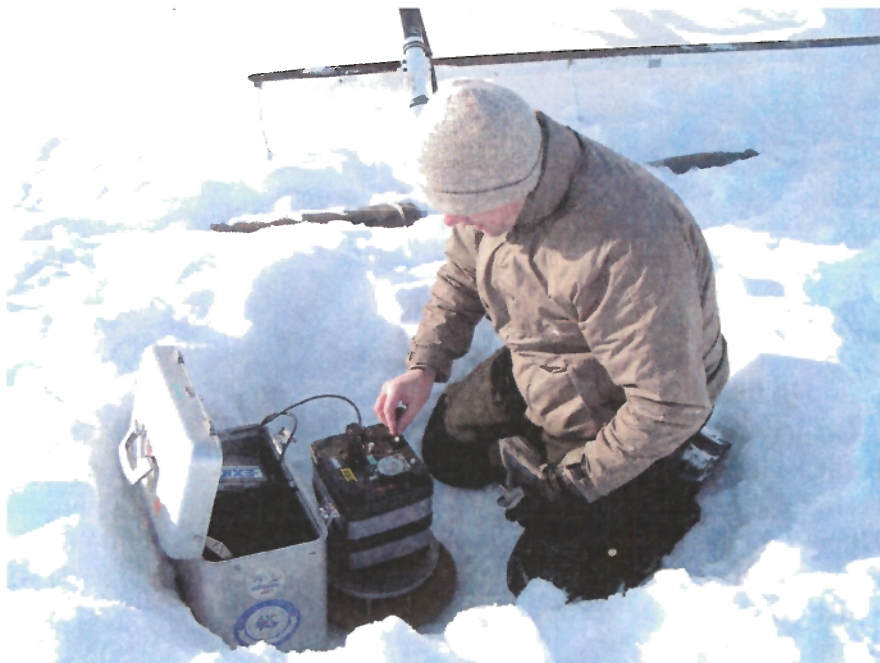
Ice camp testing - Reson NS420DS echo sounder and Knudsen 320A echo sounder
