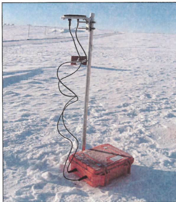
Figure 1: Cartenav ETS-1500 satellite beacon installed at the test site, 30 m south of the Spinnaker building.
