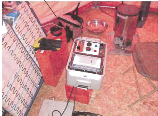
Ice camp testing - Reson NS420DS echo sounder and Knudsen 320A echo sounder
