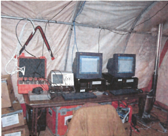
Shows one side of the electronics tent. MITS controller. Regulus computer. EPC recorder.
