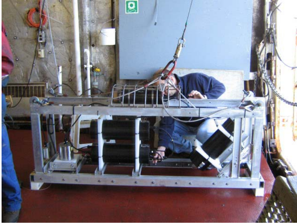
Figure 11: Close-up view of the bottom camera in the winch room.
