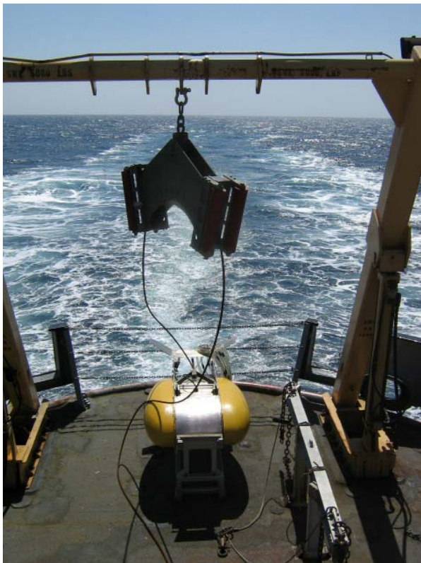
Figure 4: Huntec DTS system in its cradle, with block and A-frame above.
