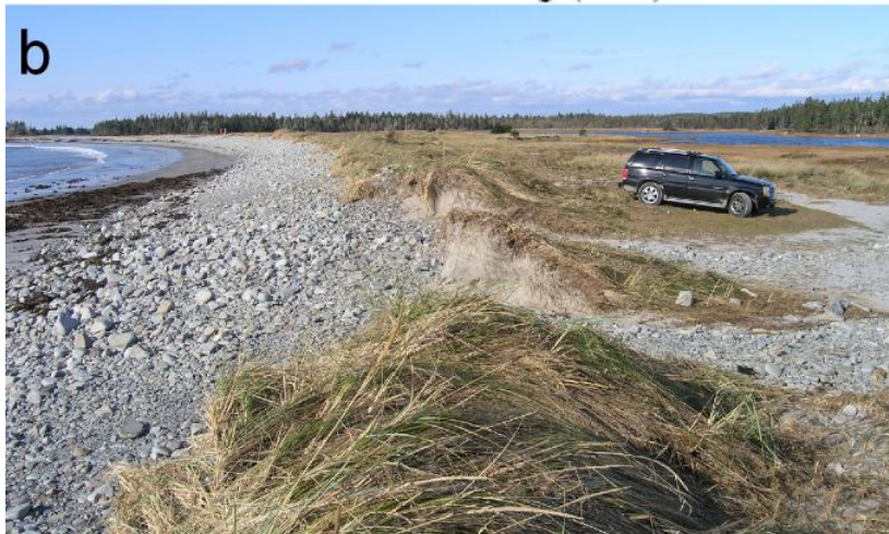
Figure 45. View and graphs of east end of Cherry Hill Beach showing changes to primary dune crest as a consequence of wave attack during Noel, Nov. 4, 2007. (a) positional changes in the dune crest since 2003 (following Hurricane Juan) and after Noel; largest landward migration was at the west end of the survey whereas at the east end beach ridges built seaward of the dune. (b) two channels cut through the dune at the main parking area. Location of parking area is shown on graphics a and c. (photo PB090612, Nov. 9, 2007, R. Taylor) and (c) longshore profile of dune crest showing the areas of greatest lowering and scouring and the small area that remained intact- To better understand this profile pretend you are standing offshore looking back at the beach looking at the highest part of the beach which consists of many low areas cut by waves.
