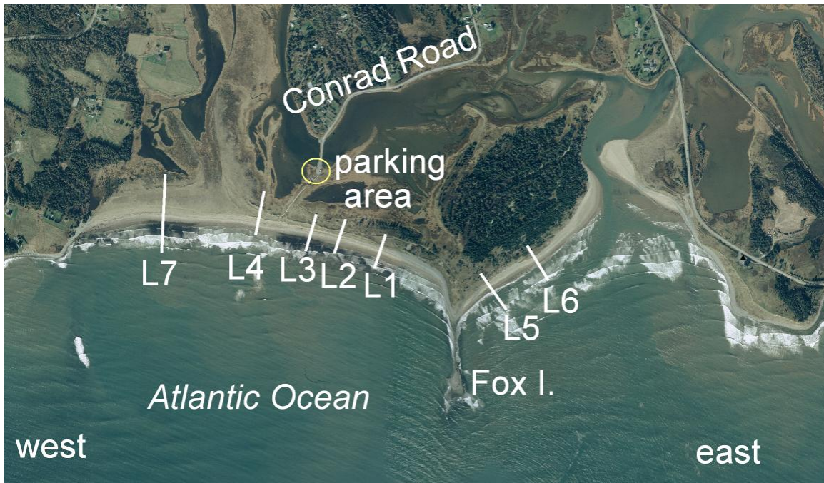
Figure 9. Location map of cross-shore survey lines 1 to 7 established on Conrads Beach in the 1980s. Lines (L) 2 and 4 were resurveyed following Post-tropical Storm Noel on Nov 6, 2007. (Digital 2003 air photo 4460633 & 4465633, courtesy NS Department of Natural Resources).
