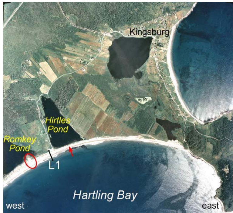
Figure 38. Aerial view of Hirtles Beach at the head of Hartling Bay showing the location of survey line L1, the new channel cut through the beach during Noel (arrow) and site of the tidal channel (circle) that flows into Romkey Pond (air photo 92354-143; July31,1992).
