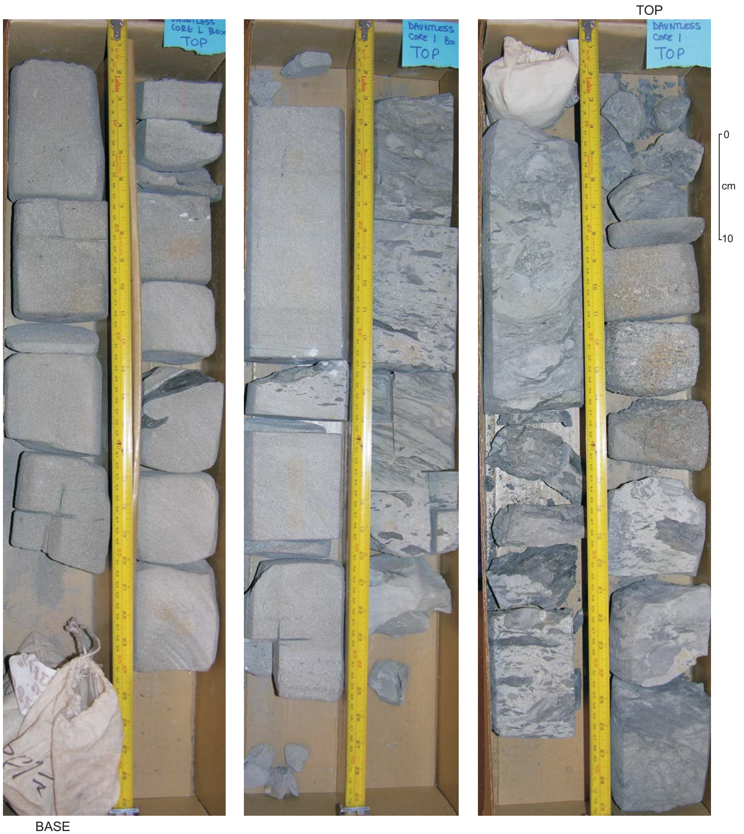
Figure 4: (a) Photographs of core 1, sandstone and minor shale, Missisauga Formation, Dauntless D-35, 3162.6-3172.1 m.
